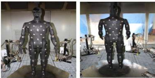
[1. The instrumented manikin of SENAI-CETIQT (front view on left and backview on right).]
