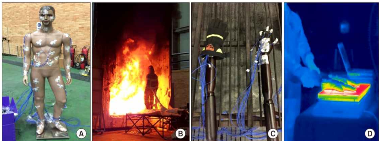
[ 1. Experimental settings of real scale fire test and hot plate test. (A) heat flux gauge, body of manikin. (B) real scale fire test. (C) heat flux gauge, hand of manikin. (D) hot plate test. ]
