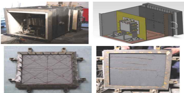
[1. Schematic diagram and view of experimental chamber and Thermocouples and sample-holder.]
