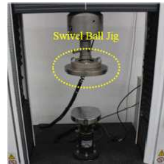
Compressive test set up with swivel ball type jig
